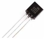
Fig.5. NPN bipolar transistor.
