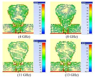
Fig. 7. Simulated current distributions of the investigated antenna at 4 GHz, 8 GHz, 11 GHz and 13 GHz
