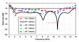
Fig. 4. Predicated return loss arcs with various numbers of W parameter
