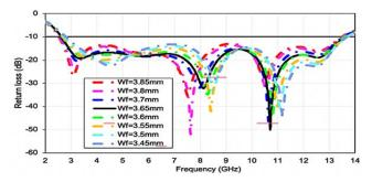
Fig. 5. Simulated return loss curves with different numbers of Wf parameter
