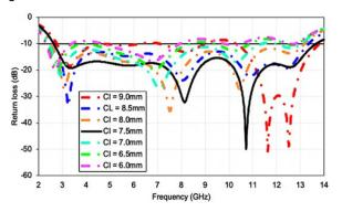
Fig. 2. Predicated return loss arcs with various numbers of CI parameter
