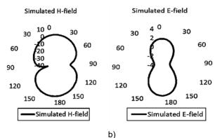
Fig. 9. H-field and E-field radiation patterns of the planar monopole antenna with CPW fed at (a) 2.911 GHz, and (b) 7.74 GHz.
