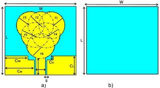
Fig. 1. The design geometry of the UWB planar antenna; (a) front look, (b) back look
