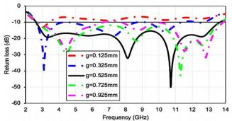
Fig. 6. Predicated return loss arcs with diverse numbers of g parameter.
