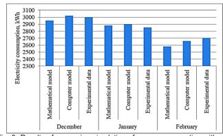
Fig. 9. Results of comparing simulation of power consumption with experimental data
