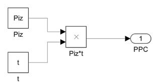
Fig. 3. Input load simulation control unit
