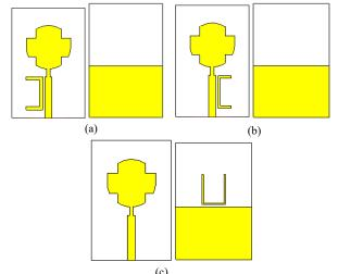
Fig. 2. Schematic diagram of the development for proposed monopole antenna with U-shaped element (a) Antenna B1 (b) Antenna B2, (c), Antenna B3
