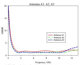
Fig. 7. VSWR of the for the proposed monopole antenna of Antenna A1, Antenna A2 and Antenna A3
