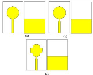
(c) Fig. 1. Schematic diagram of the development for proposed monopole antenna (a) Antenna A1 (b) Antenna A2, (c), Antenna A3
