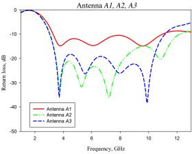
Fig. 4. Return loss of the for the proposed monopole antenna of Antenna *A1*, Antenna *A2* and Antenna *A3*
