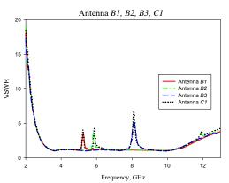
Fig. 8. VSWR of the for the proposed monopole antenna of Antenna *B1*, Antenna *B2*, Antenna *B3* and Antenna *C1*
