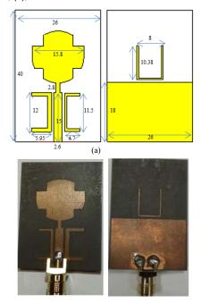
Fig. 3. Schematic diagram of the development for proposed monopole antenna of Antenna *C1* with combined three U-shaped elements, (a) simulation, (b) fabricated
