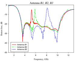
Fig. 5. Return loss of the for the proposed monopole antenna of Antenna *B1*, Antenna *B2* and Antenna *B3*
