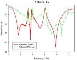
Fig. 6. Return loss of the for the proposed monopole antenna of Antenna C1 (simulation vs measurement)
