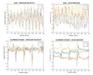
Fig. 5. MPU6050 sensor indications while running and climbing stairs
