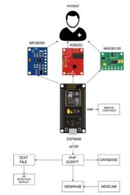
Fig. 3. Wiring diagram of the developed system
