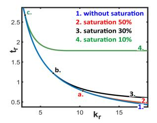
Fig.5. The dependence of the settling time  $t_r$  on  $k_r$  for control systems with and without saturation
