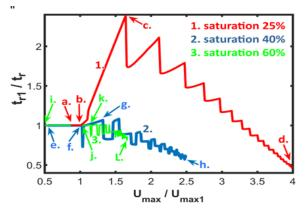
Fig.12. Relative control quality indicator for  $t_r$  for saturation  $U_{maxl}=25\% U_{max}$ ,  $U_{maxl}=40\% U_{max}$  and  $U_{maxl}=60\% U_{max}$
