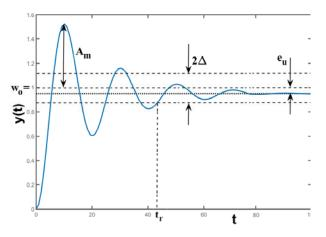
Fig.2. Output signal y(t) with marked parameters  $A_m$ ,  $t_r$ , and  $e_u$
