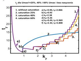
Fig.10. The dependence of the settling time  $t_r$  on  $k_r$  for control systems with and without saturation
