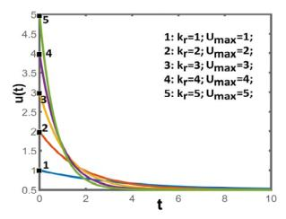
Fig.4. Control signal u(t) for various values of  $k_r$
