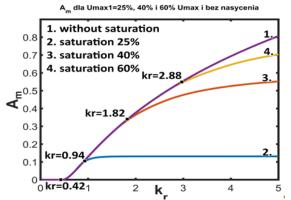
Fig.11. The dependence of the overshoot  ${\cal A}_m$  on  $k_r$  for control systems with and without saturation
