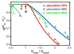
Fig.13. Exponential control quality indicator for  $A_m$  for saturation  $U_{maxl}=25\% U_{max}$ ,  $U_{maxl}=40\% U_{max}$  and  $U_{maxl}=60\% U_{max}$
