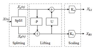
Fig.1. The lifting scheme
