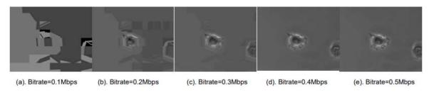
Fig 5. The decoded frames using the BANDELET (LIFTING)+SPIHT algorithm at each bitrate
