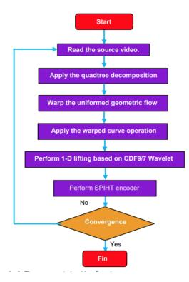
Fig.3. The proposed algorithm flowchart steps
