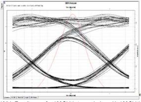
Fig.10(b). Eye diagram for 100Gbit/s transmission with 100Gbit/s
