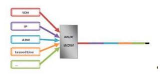
Fig.2. Principe Multiplexing with different protocols
