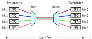
Fig.1. Schematic of a WDM system
