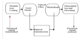
Fig.4. Optical fiber transmission chain
