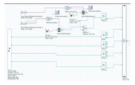
Fig.11(a). 100Gbit/s WDM system transmitted component with ROADM architecture in 200Km length FO
