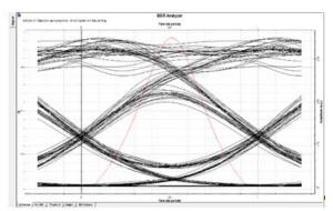
Fig.10(c). Eye diagram for 100Gbit/s transmission with 110Gbit/s
