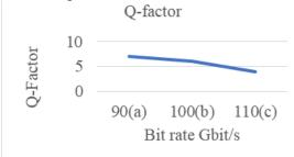
Fig.12(b). Effects of FO length and Bit rate on Q-Factor
