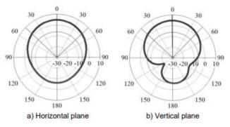
Fig. 8 2D radiation pattern from simulation of the trapezoidal patch with a multi-slot antenna
