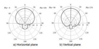
Fig. 3. 2D radiation pattern from the simulation result of the rectangular patch antenna
