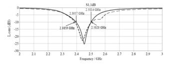
Fig. 10. S11 measurement and simulation results for trapezoidal patch antenna with multi-slot
