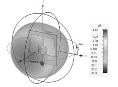
Fig. 7 3D radiation pattern from simulation of the trapezoidal patch with a multi-slot antenna
