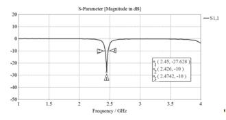
Fig. 2. S11 from simulation results of regular rectangular patch antenna
