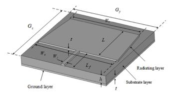
Fig. 4. A trapezoidal patch antenna model
