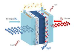
Fig.1. Schematic of PEM fuel cell operation
