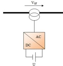
Fig.3. Series active power filter
