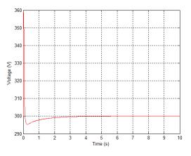
Fig.11. DC link of inverter
