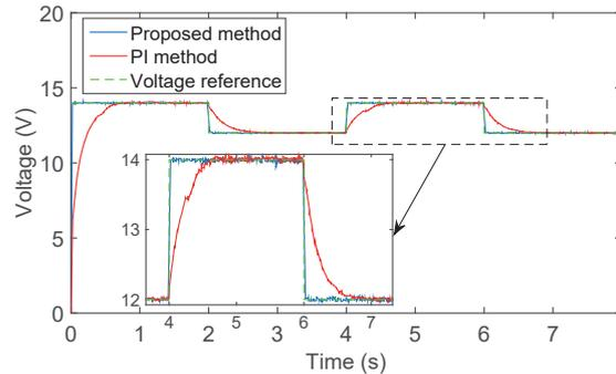
Fig. 13. Comparison between FLC and PI controllers.
