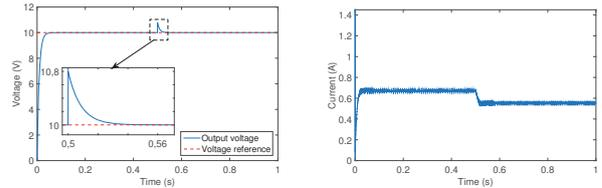
Fig. 7. Simulation results for a voltage reference  $V_{ref} = 10V$  and variable load.
