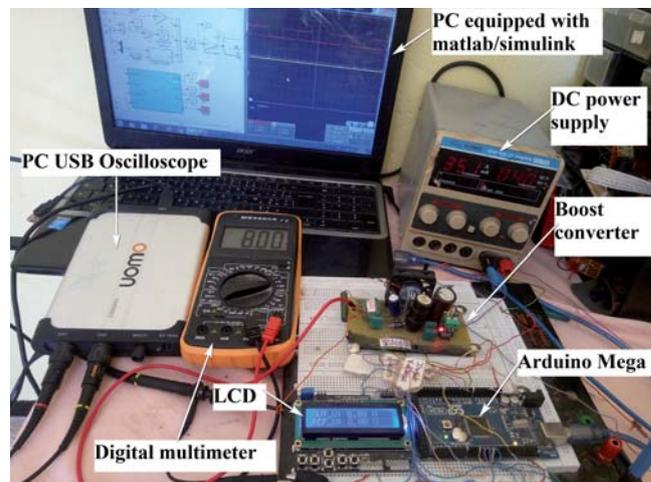
Fig. 9. FLC Hardware implementation using Arduino Mega and Matlab/Simulink environment.
