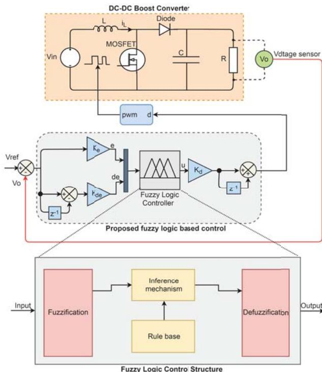
Fig. 1. Proposed FLC structure for boost converter.
