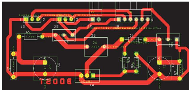
Fig. 3. Boost converter PCB.
