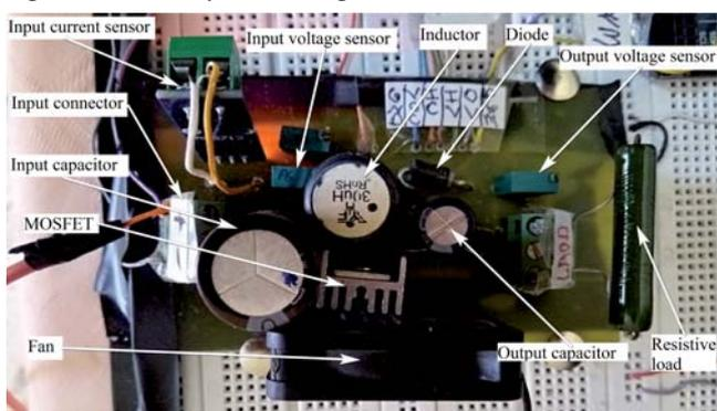
Fig. 2. Boost converter prototype.
