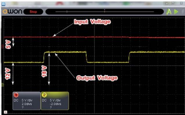
Fig. 12. Results recorded using PC USB oscilloscope.
