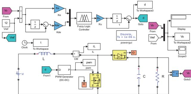
Fig. 5. DC-DC boost converter with FLC.
