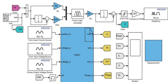
Fig. 8. Simulink model used to implement the FLC.
