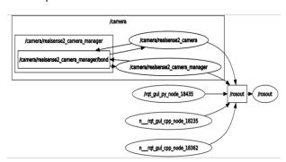
Fig.4. Rqt graph of nodes and topics for camera and Raspberry Pi in ROS.
