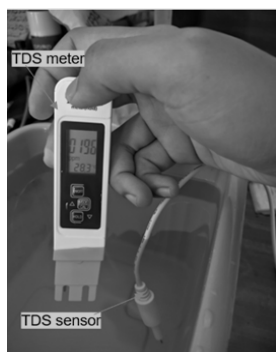
Fig.8. TDS meter and TDS sensor
