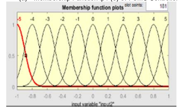
(b) Membership Function ip2 (e) of FSMC Controller
