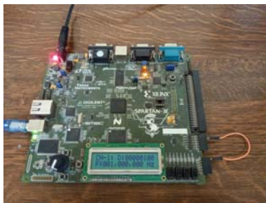
Fig. 15: Input frequency (1MHz) to Channel_1
