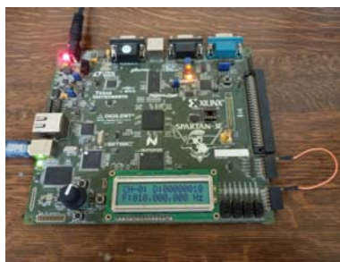
Fig. 11: Input frequency (10MHz) to Channel_0
