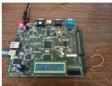
Fig. 12: Input frequency (10KHz) to Channel_0
