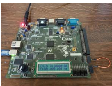
Fig. 17: Input frequency (1MHz) to Channel_3
