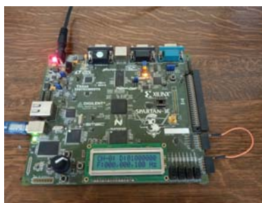
Fig. 14: Input frequency (100Hz) to Channel_0
