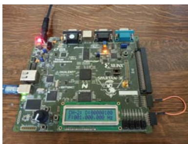
Fig. 16: Input frequency (1MHz) to Channel_2
