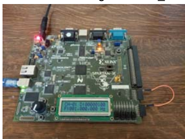
Fig. 10: Input frequency (1MHz) to Channel_0
