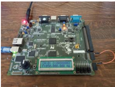
Fig. 8: Input frequency (50MHz) to Channel_0
