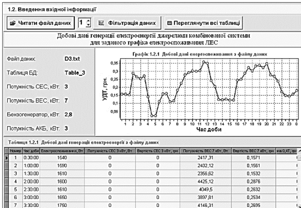
Fig. 5. Interface for entering the output data of the software module of dynamic energy management CES with a wind-solar system, gasoline power station and static power supply.
