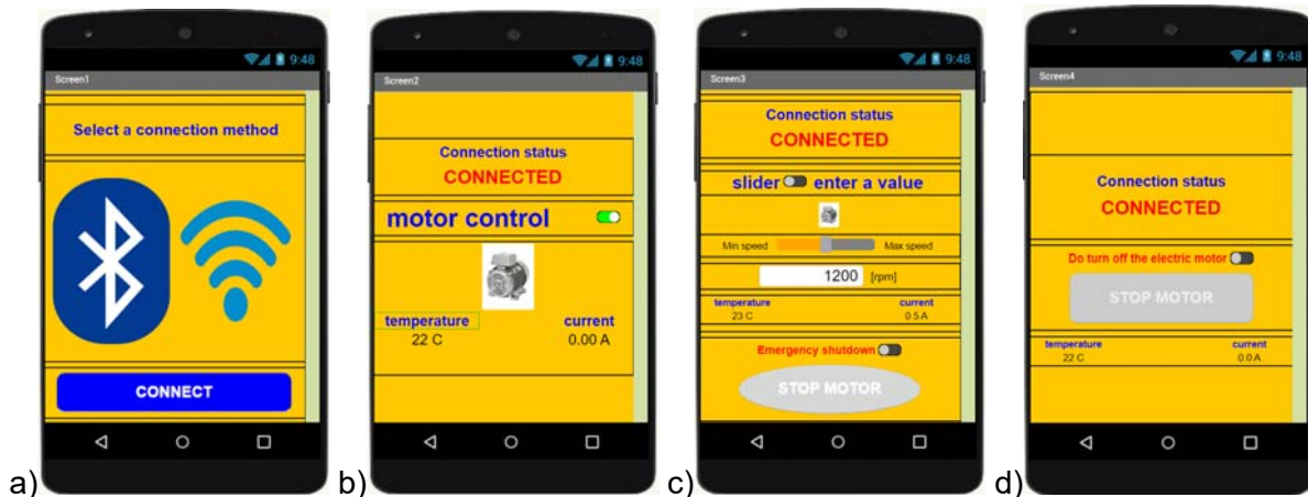
Fig.2. The interface of the developed mobile application with sequentially switched screens; from the left: a) Establishing a connection (Bluetooth or Wi-Fi); b) Enabling control; c) Motor rotational speed control (using a slider or entered value) with an emergency stop; d) Motor shutdown and disconnect
