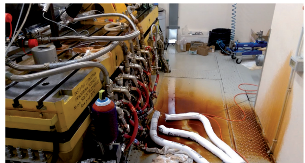
Fig. 2. Example of oil leakage in component test laboratory
