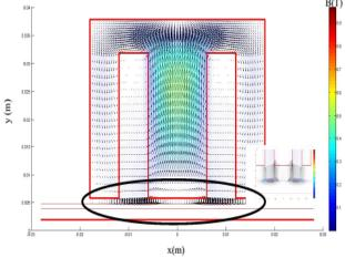
Fig. 8.c. 2D distribution of magnetic field vectors and magnetic induction for f= 150kHz.
