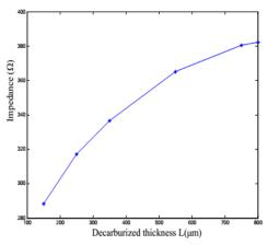
Fig. 7. Impedance values calculated at 1 kHz frequency for various decarburized layer thicknesses L = [150-800]µm.
