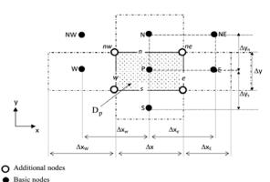
Fig. 3. Projection of the elementary volume according to the XY plane.
