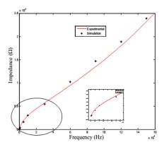
Fig. 5. Computed and measured impedance profile via frequencies (f = 50Hz-150 kHz) for a specimen with decarburized layer thicknesses L = 200  $\mu$ m.
