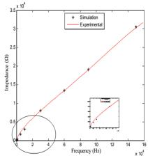
Fig. 4. Calculated and measured impedance profile via frequencies (f = 50Hz-150 kHz) for a specimen with decarburized layer thicknesses L = 800  $\mu$ m.
