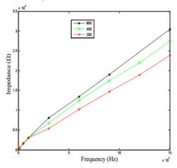
Fig. 6. Calculated impedance profile via frequencies(f = 50Hz-150 kHz) for a specimen with decarburized layer thicknesses L = 800  $\mu$ m, L = 400  $\mu$ m and L = 200  $\mu$ m.
