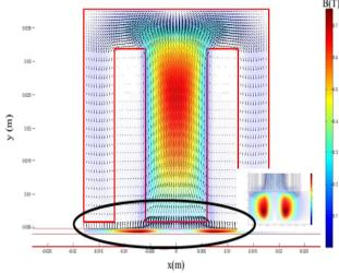
Fig. 8.b. 2D distribution of magnetic field vectors and magnetic induction for f= 1 kHz.
