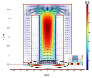
Fig. 8.a. 2D. Distribution of the magnetic field vectors and magnetic induction values for  $f=50\,\text{Hz}.$
