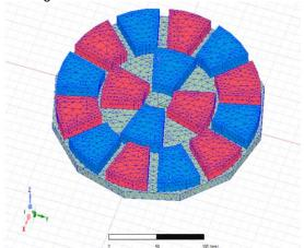
Fig. 2 Mesh of magnetic disk
