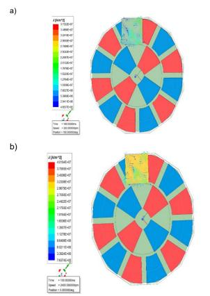
Fig. 4 Eddy current in 3D rectangular copper particle: (a) 300 Rpm, (b) 2400 Rpm
