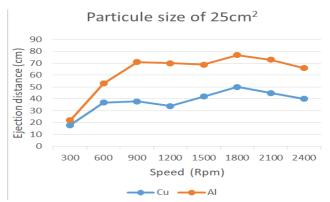
Fig. 8 Ejection distance of non-ferrous particles
