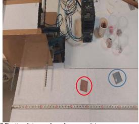
Fig. 7 Ejection distance of non-ferrous particles
