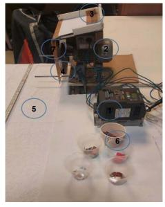
Fig. 6 Setup of magnetic separation device 1-Driving motor command 2-Motor 3-Feeder 4-Permanent magnet disk 5-Collectors of fall particles 6- Particles waste 7-Plastic Isolation
