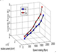
Fig. 5 Induced current and ejection force on two types of rectangular non-ferrous particles
