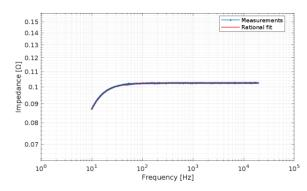
Fig. 12. Approximation of the SCT013 current transformer frequency characteristic for NPoles = 2 in a limited frequency range
