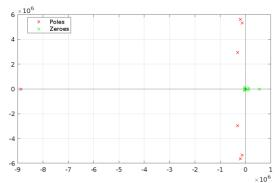
Fig. 9. Zeros and poles of the impedance of the SCT013 transformer shown on the complex plane.
