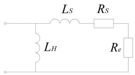
Fig. 3 One-phase model of current transformer
