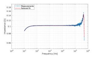
Fig. 10. Approximation of the SCT013 current transformer frequency characteristic for NPoles = 4 in a limited frequency range.
