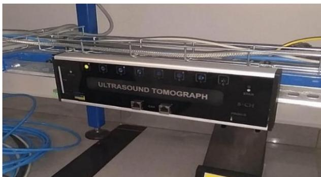
Fig. 2. Semi-industrial ultrasonic tomography workstation - tomograph PCB with cover adapted to DIN13 connector.
