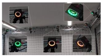
Fig. 13. Motion capture system with visible LED rings of Prime<sup>x</sup> 13W cameras; the orange colour indicates that a camera has not yet reached operating temperature.
