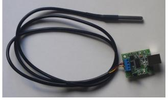
Fig. 14. DS18B20 thermometer and 1-wire to USB converter module; the data from the thermometer can be read directly in an application written in C/C++ programming language.
