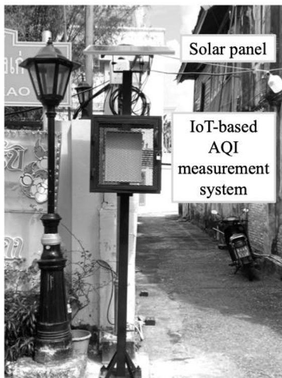
Fig. 2. Actual hardware setup of the deployed IoT-based AQI monitoring system.
